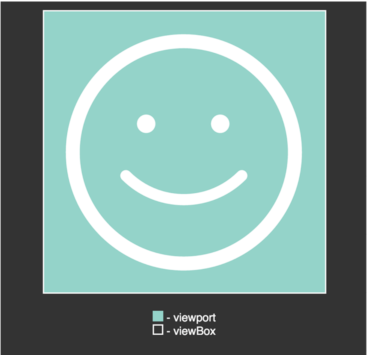
FIG 6.2: With the viewport enlarged and viewBox kept the same, the graphic scales up to fit the viewport.
